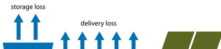
Irrigation water is released from the storage and transported to farms via natural water courses (for example rivers) and irrigation channels. Losses occur both in storage and in the delivery of water through evaporation and seepage. It is assumed there exists no on farm storage and no in stream or tributary flows downstream of the storage.
